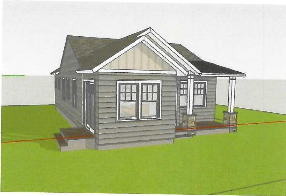
View of Side Entry- Steps and Roof Overhang that require a Side-Yard Variance
