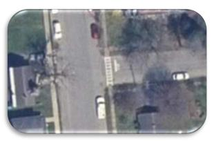
Ford St and Thompson St - This 4-legged intersection has all-way stop sign control. There are no sidewalks at the intersection, or striping pedestrian crosswalks. Each approach at this intersection has a single inbound and single outbound lane. The St. Mary's School is just south of this location and a 15 mph school speed limit starts immediately south of this intersection.
