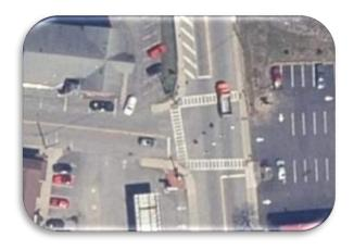
parking is set-back from the intersection, so it generally doesn't impact intersection operations. The signal operates with two phases, one for mainline Milton Ave, the other for the side street/driveway.
