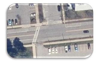
Bath St and Front St - This 4-legged intersection is traffic signal controlled. It has one through lane in each direction, and crosswalks across each approach, but no pedestrian signals. The signal is old and doesn't meet current design standard, but appears to operate acceptable in a fixed time mode (same timing every cycle regardless of the presence of traffic). The signal operated with two phases, on for the Bath St approaches, the other for the Front St approaches.
